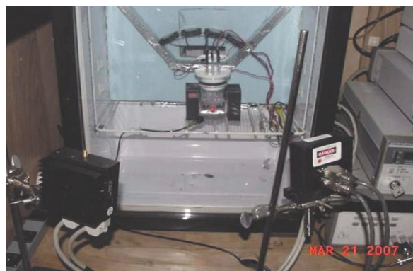
Figure 2. Cell inside a temperature enclosure designed to hold ambient temperature at 25 \pm 0.03^\circ\text{C} . A pair of permanent magnets is positioned next to the cell and provides approximately 625 gauss at the cathode. The dual lasers are shown in the foreground.
